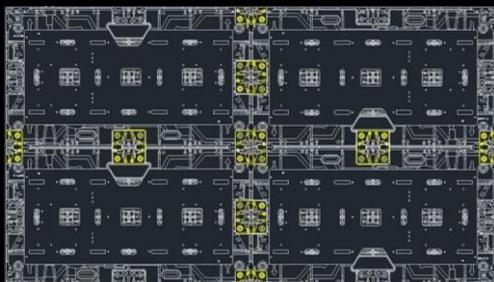
Block connector system (shown in yellow squares above) on the cabinets allow for self-corrective seamless alignment.
