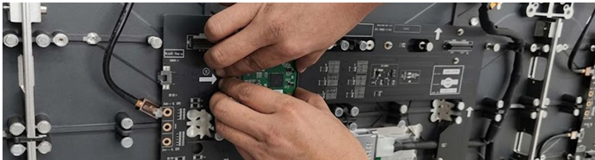
Pay attention to the direction of receiving card when installing the receiving card
