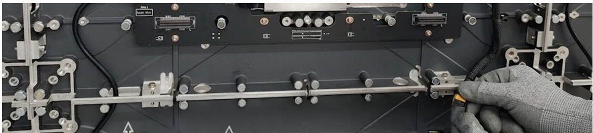
Remove the fixing screws of the HUB board
